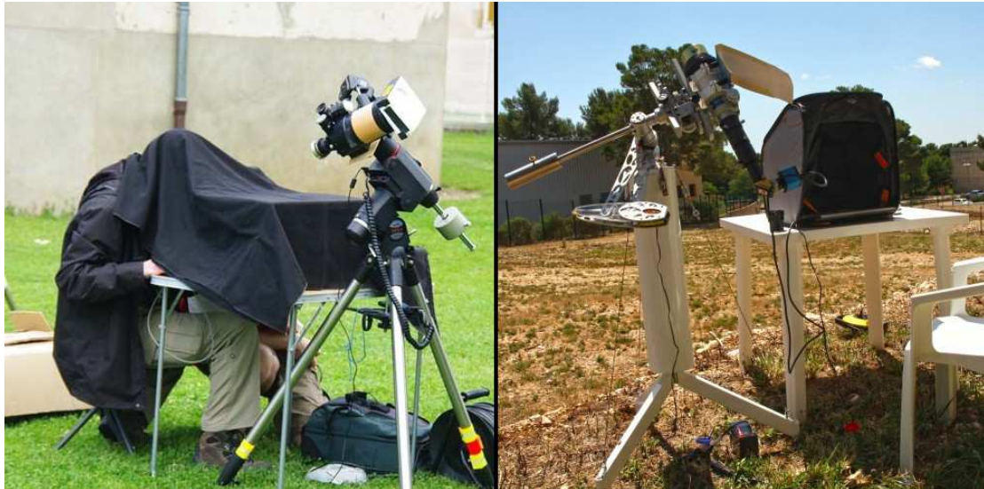
Fig. 3 Distinguishing poor surface contrast requires the best possible viewing conditions. Left, a homemade dark room (Photo by J-P Godard); right, a commercial shadowing tent.
