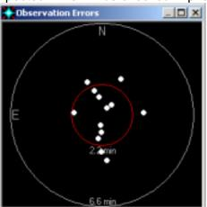
The two circles are the 1-sigma and 3sigma error circles. The red inner circle contains about 68% of the observations, and the white outer circle contains approximately 99% of the observations. The text displayed at the bottom of each circle gives their diameters in arc-minutes.
